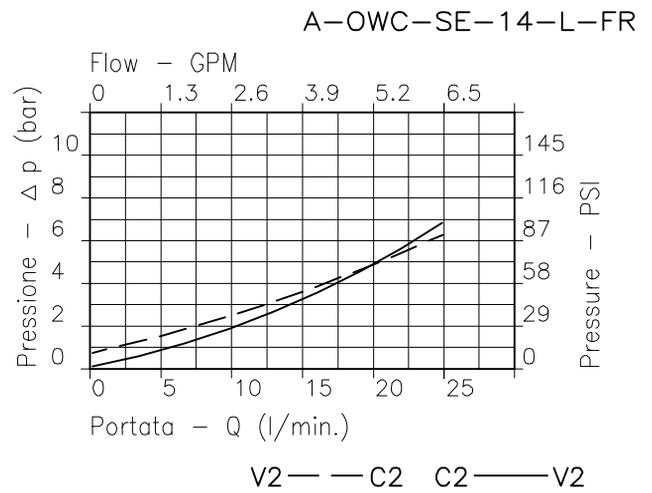
**Viscosità olio 46 cSt a 50°C - Oil viscosity 46 cSt at 50°C**
